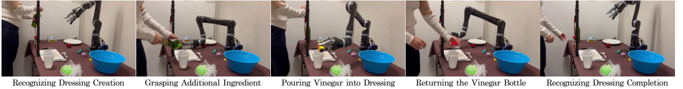
Fig. 4: Example of our assistive HRC system: Shortly after the user starts to prepare the dressing, the robot identifies the intention and correctly assists the user in creating the dressing by adding further ingredients.
